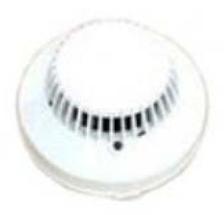
The Salwico DOS3 (N1115) is a low profile conventional Optical Smoke Detector designed to combine optimal response to smoke with a strong immunity to false and unwanted alarms. The sensor employs an alarm verification function which requires two successive pulses before an alarm is given.
